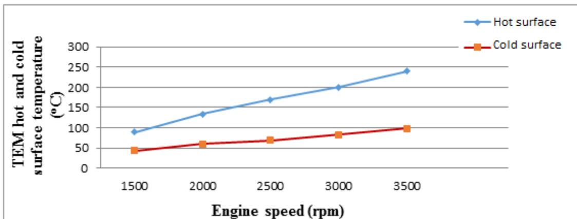
Figure 4. The temperatures on the surface of TEM
