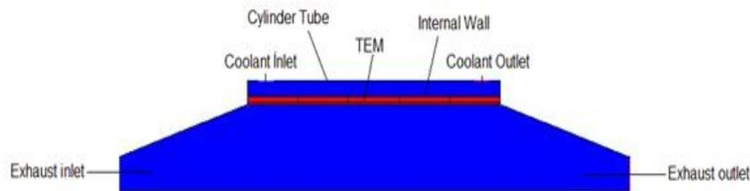
Figure 2. Two-dimensional view of the TEG System
